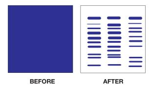
3. A single CoZap pad may be used for several gels and may be left in the destaining solution for the next usage. When the CoZap pad turns a deep blue color, replace the pad. It is not necessary to change the destaining solution when replacing the CoZap pad.
